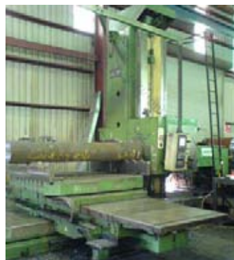
Union CNC 6 axis horizontal borer with 2,700 cross x2,500 vertical x2,300 long travels, full contouring B axis 2000 x 1800 table size & 8,000Kg table capacity. Includes a programmable facing head suitable for boring to 1400mm diam.
