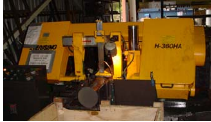
Auto feed bandsaw suitable for cutting up to 360mm diameter bar.
